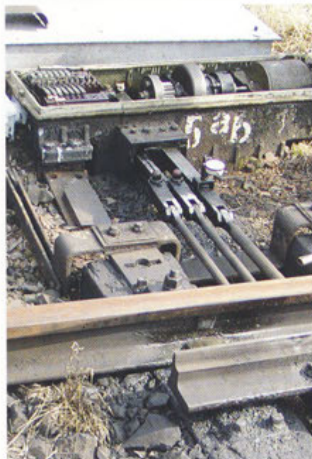
Fig. 1a): Plunger measurement: plunger location (a white element on the point rod, between the point machine and rail)
