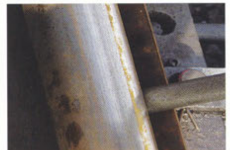
Fig. 1c): Obstacle between a stock rail and switch blade
