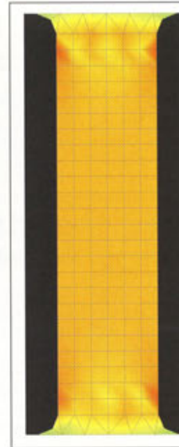
Fig. 7b): Equivalent deformations in the measuring element
