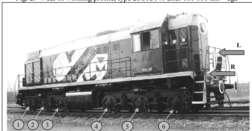
Fig. 3 TEM2 locomotive, as well as distribution and numeration of tested wheelsets
