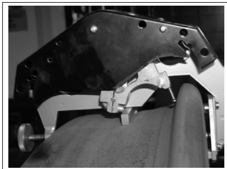
Fig. 1. ‘A-B profilometer’ for railway wheel tyres
