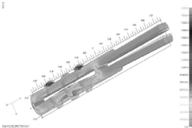
Fig.3 The map of strain with maximum dislocation of EZK measurement slotted pin elements made in NASTRAN program
