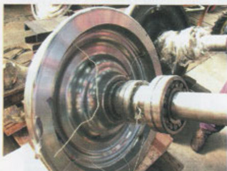
Fig. 34. Placing of thermocouples along the wheel circumference (9 mm away from the rolling surface)
