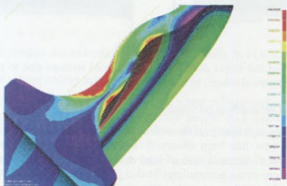
Fig.17. Stress superposition for PN 920/200s wheel
