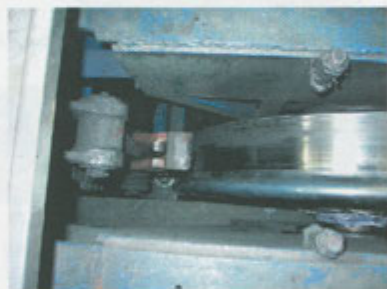
Fig.32. Test stand for deformation and temperature investigation of railway wheelsets wheels
