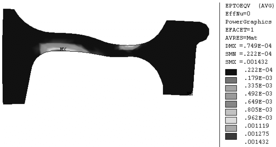
Fig. 8. Distribution of the given complete deformations by VonMises criterion \sigma_{mst} at the moment of time B
