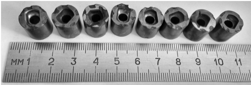
Fig. 5. Defects of cylindrical cutting tools
