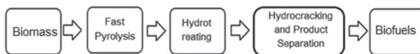
Figure 1 Scheme of converting biomass into liquid fuels by upgrading the bio-oil Slika 1. Prikaz pretvaranja biomase u tekuća goriva poboljšanjem bionafte
