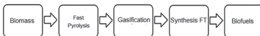
Figure 3 Scheme of the Gasification Process of Biomass on Liquid Fuels Slika 3. Prikaz procesa uplinjavanja biomase pri tekućim gorivima
