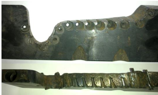
Figure 10. Tool holder with sealed cutters
