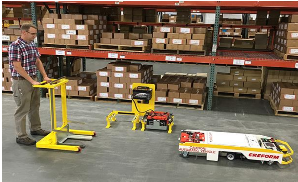
Fig. 8. Manual battery swap platform [9]
