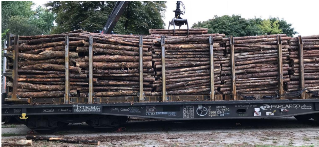
Fig. 12. Loading of timber into stanchion baskets on a platform wagon
