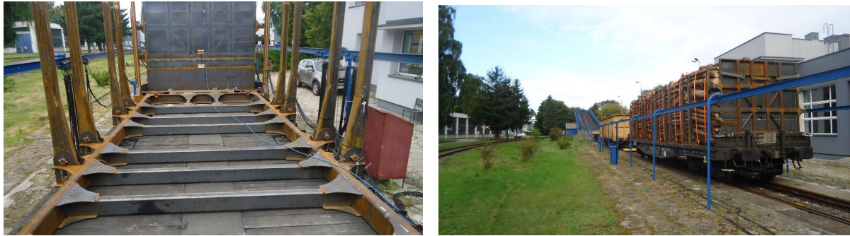
Fig. 10. Wagon and stanchion basket on Rgmms platform: (a) strain gauge installation fitted and (b) a wagon with baskets on the test bed
