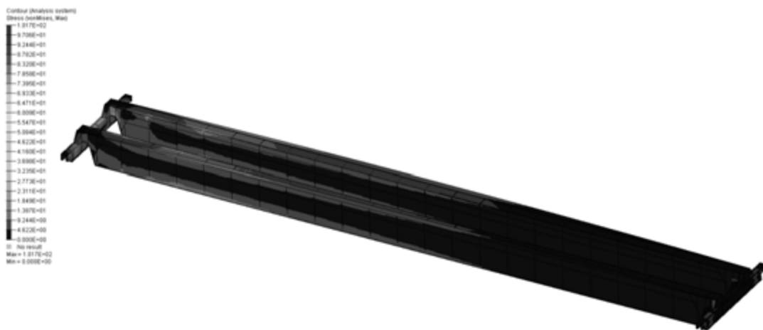
Fig. 20. Von Mises stress for structure with nominal load 200 kN without gravity effect (trolley at left side)
