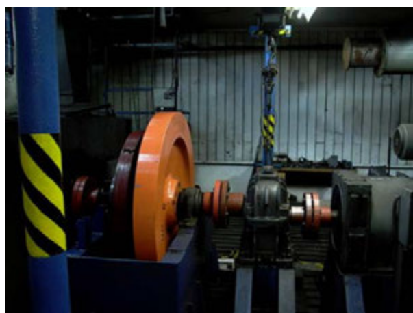
Fig. 11. Test stand for deformation and temperature investigation of railway wheelsets wheels
