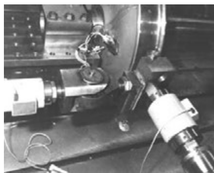
Fig. 6. Strain test stand for investigation of railway wheelsets' wheels deformations
