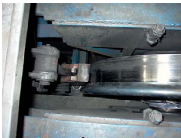
Fig. 11. Test stand for deformation and temperature investigation of railway wheelsets wheels
