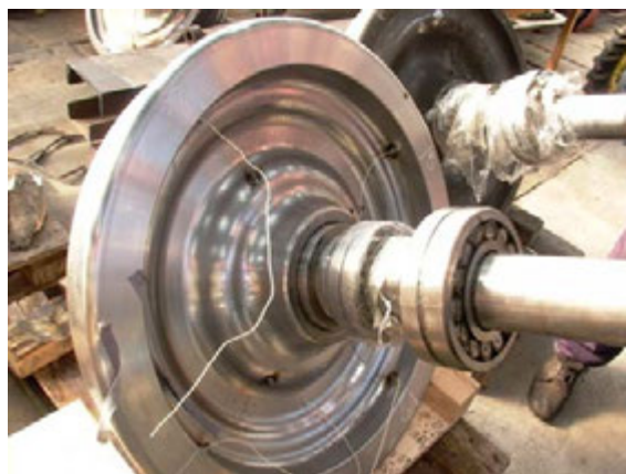
Fig. 13. Placing of thermocouples along the wheel circumference (9 mm away from the rolling surface)
