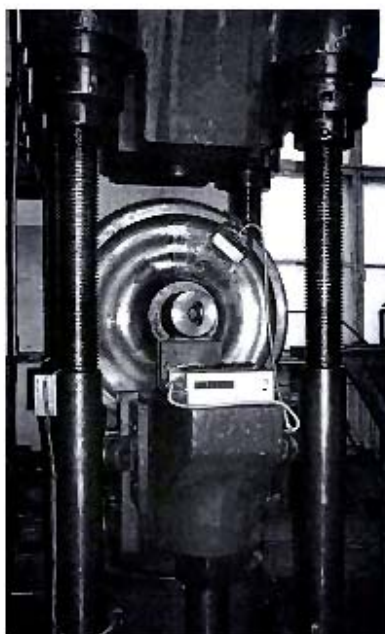
Fig. 1. Test stand for strain investigation of railway wheels deformation: a) the stand, b) placing of strain gauges, way of modelling the wheel
