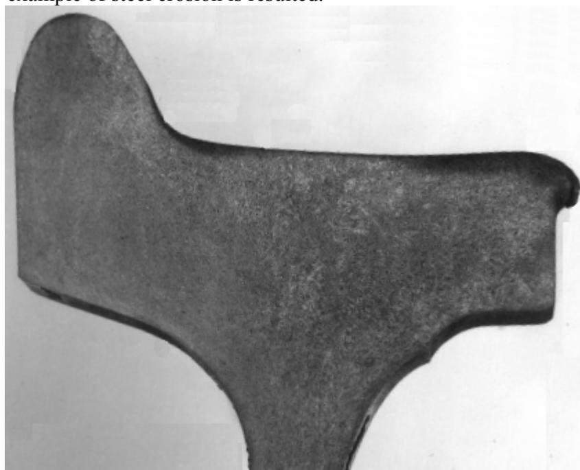
Fig. 1. Macrostructure of a wheel No 1 with the worn rim
