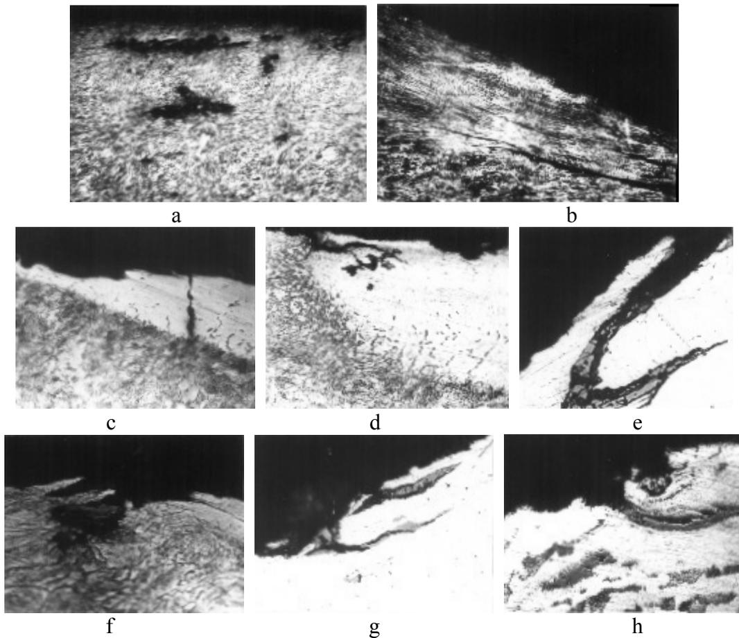
Fig. 11. Microcracks and stratifications near to a working surface
