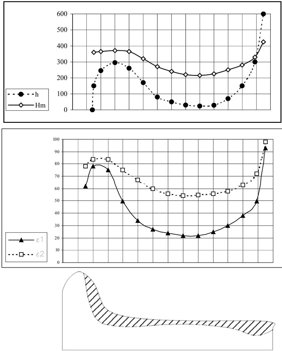
Fig. 8. Change of a degree of grains deformation across  $\epsilon_1$  and in a rolling direction  $\epsilon_2$  [%], microhardness  $H_\mu$  [ $\times 10$ , MPa] and depths of a zone of plastic deformation  $h$  [ $\mu m$ ] on width of a wheel No 1
