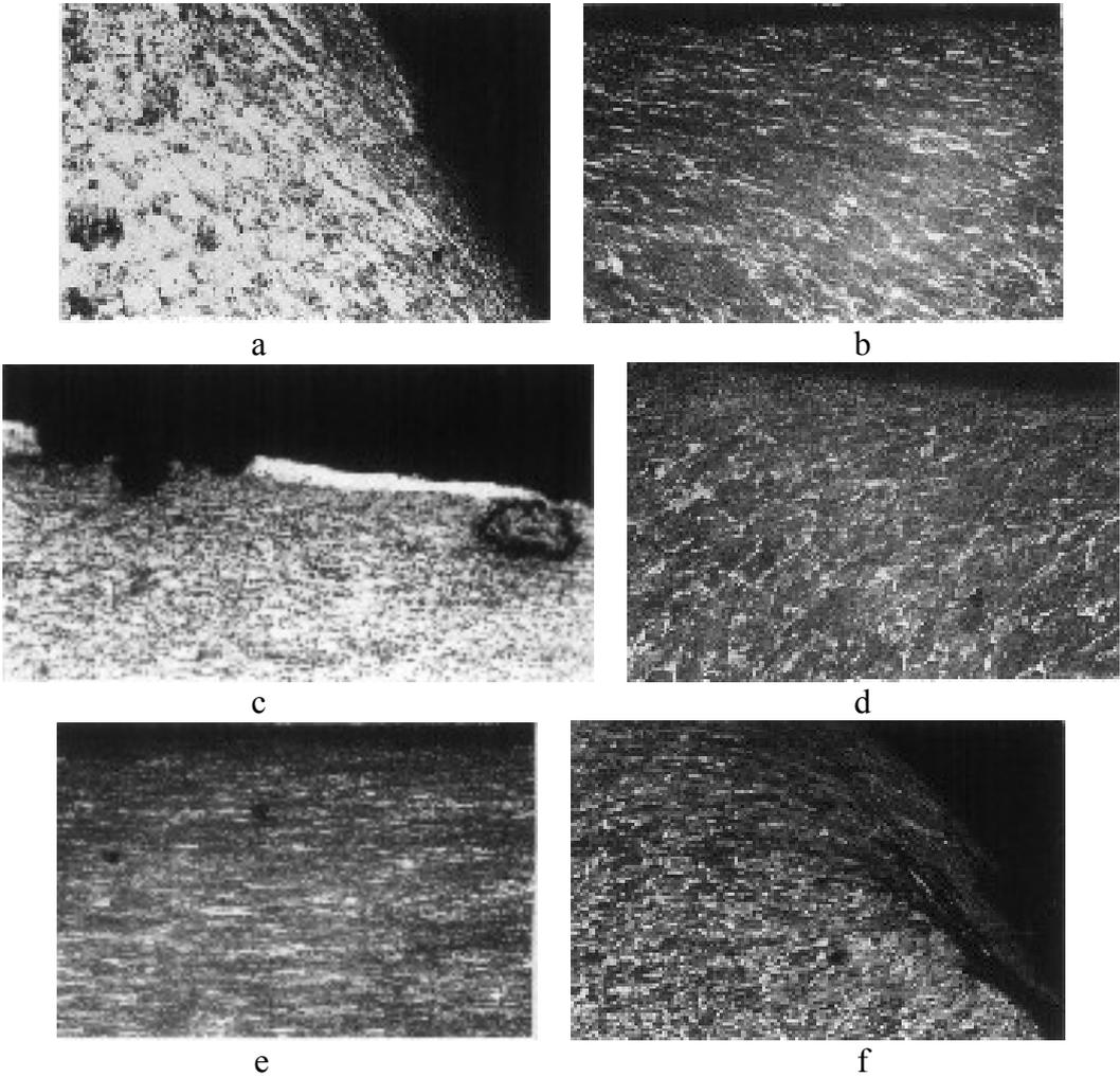
Fig. 13. The microstructure near to a working surface of the worn out rim of the wheel No 6 in a cross section, x200
