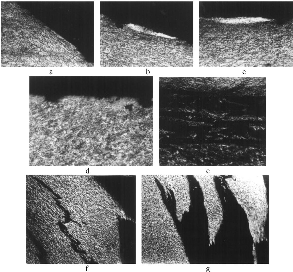
Fig. 6. The microstructure of different sites of the worn working surface of a wheel No 1; x200
