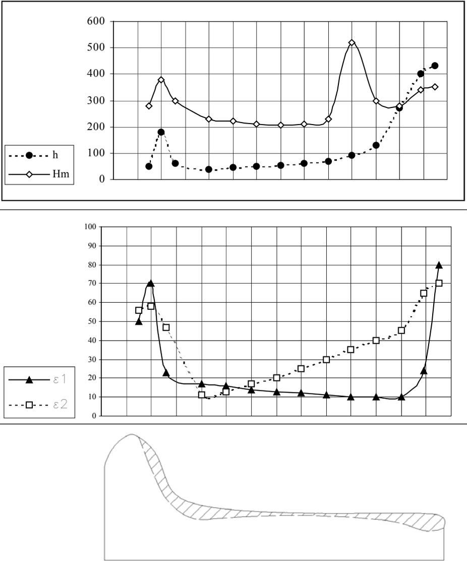
Fig. 14. Change of a degree of grains deformation across  $\epsilon_1$  and in a rolling direction  $\epsilon_2$  [%], microhardness  $H_\mu$  [ $\times 10$ , MPa] and depths of a zone of plastic deformation  $h$  [ $\mu m$ ] on width of a wheel No 6
