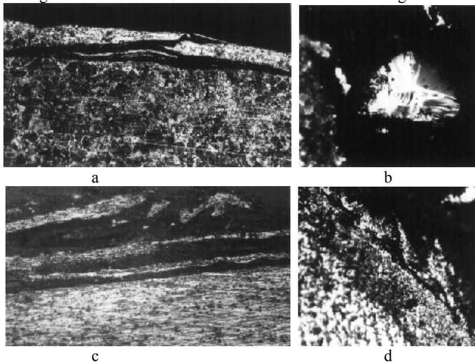
Fig. 12. The wear fragments near to a working surface
