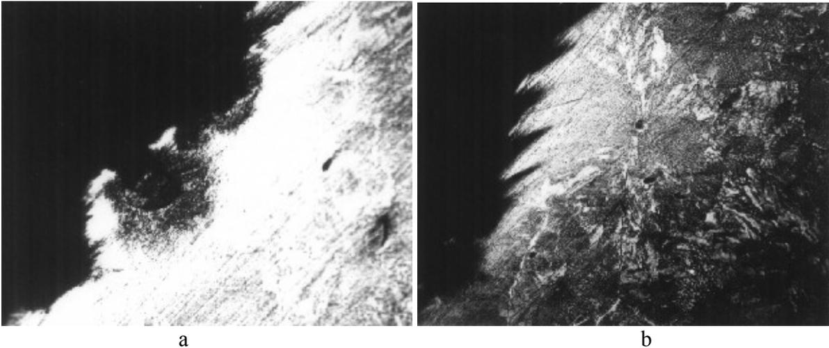
Fig. 4. Relief of a working surface of the worn rim; x200
