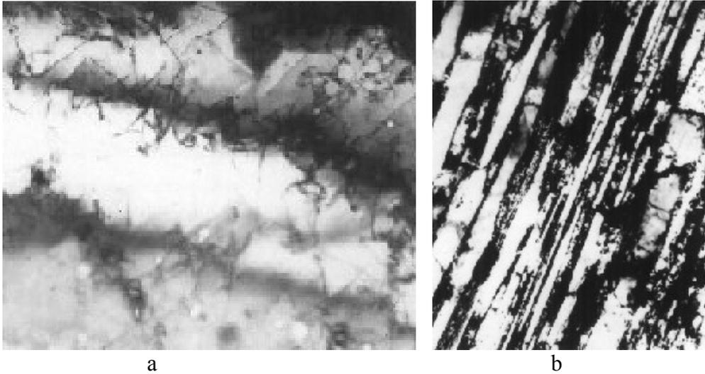
Fig. 7. The dislocation substructure of steel near to a working surface; x20000
