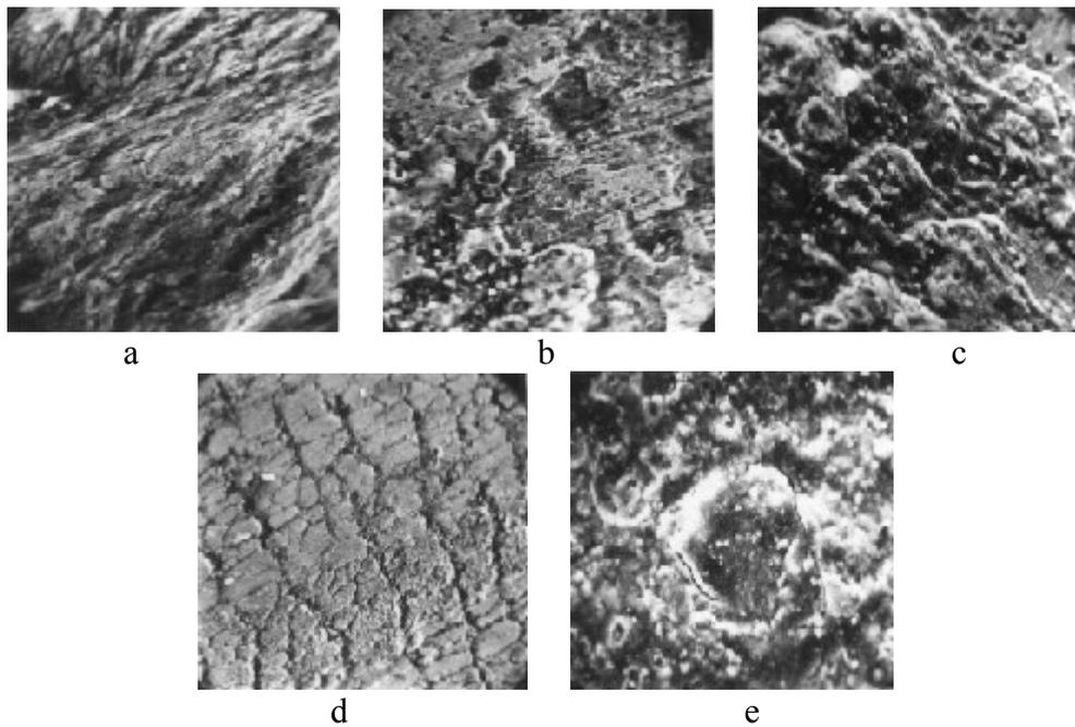
Fig. 3. Structure of a surface of a wheel 1 in different places on width of a rim; x200
