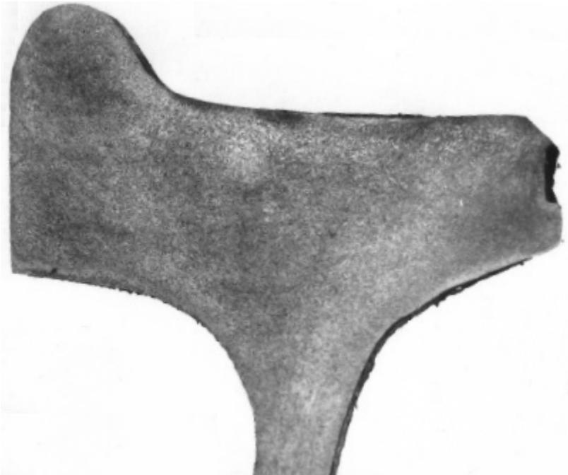
Fig. 5. Macrostructure of a wheel No 6 with the worn rim
