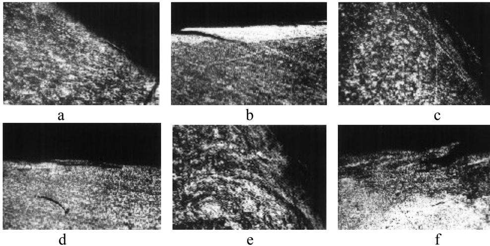
Fig. 10. The microstructure in zones of the flange gorge (a, b), the middle part (c, d) and the overflow (e, f) of wheels: No 2 (a, c); 3 (b, d); 4 (e); 5 (f); x200
