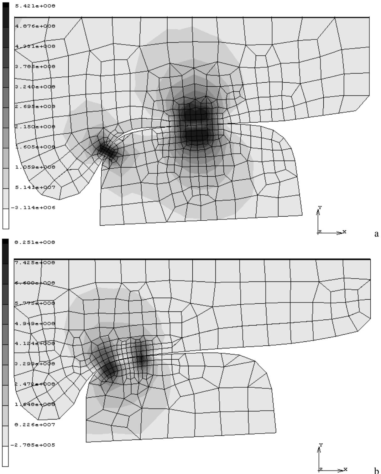
Fig. 18. The distribution of the solid Von Mises stress at the two-point contact of the rail R65 with the wheel GOST 9036-88 (a) and with the wheel DMetI (b)
