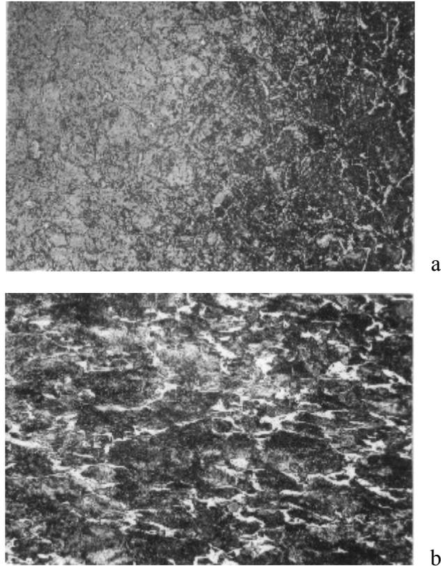
Fig. 15. The microstructure of the worn out rim of a wheel No 6 in a rolling plane; x200
