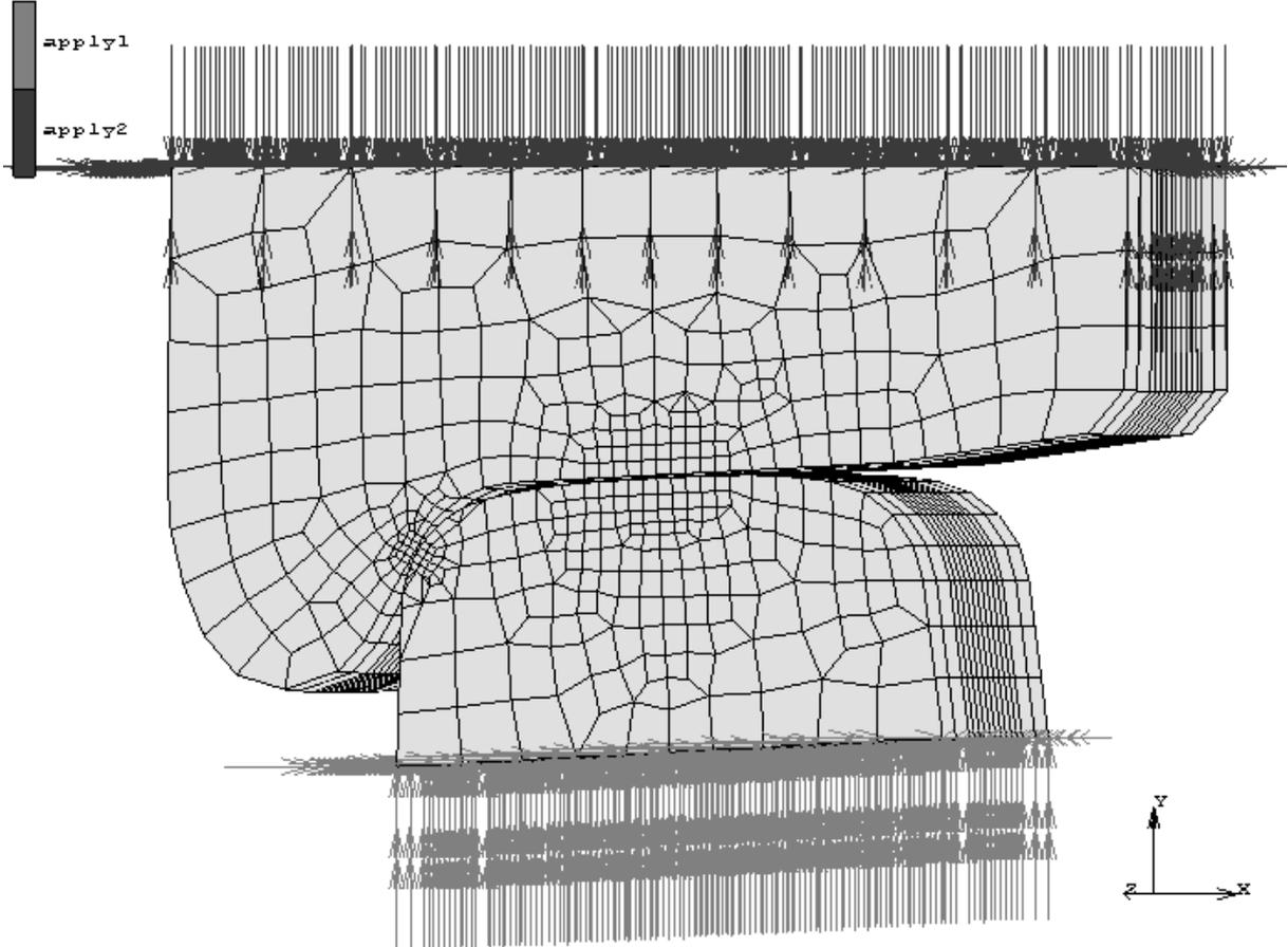
Fig. 17. An example of the coordinated FE meshes of a wheel and a rail. The boundary conditions set in the MSC.MARC software is shown also
