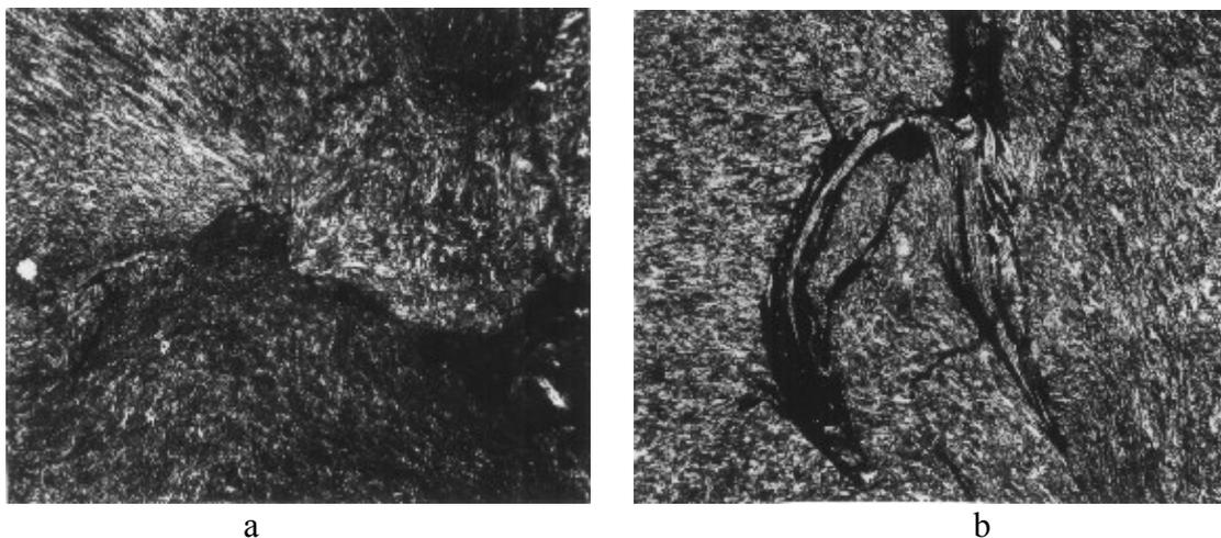
Fig. 9. The microstructure of the worn rim of a wheel No 1 in a plane determined by the tapping line; x200
