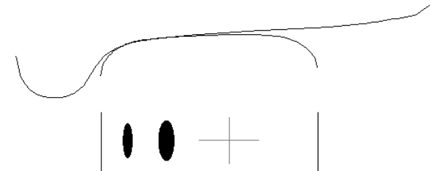
figure 10 Distribution of contact zones at contact new standard rail and wheel with new profile of surface
