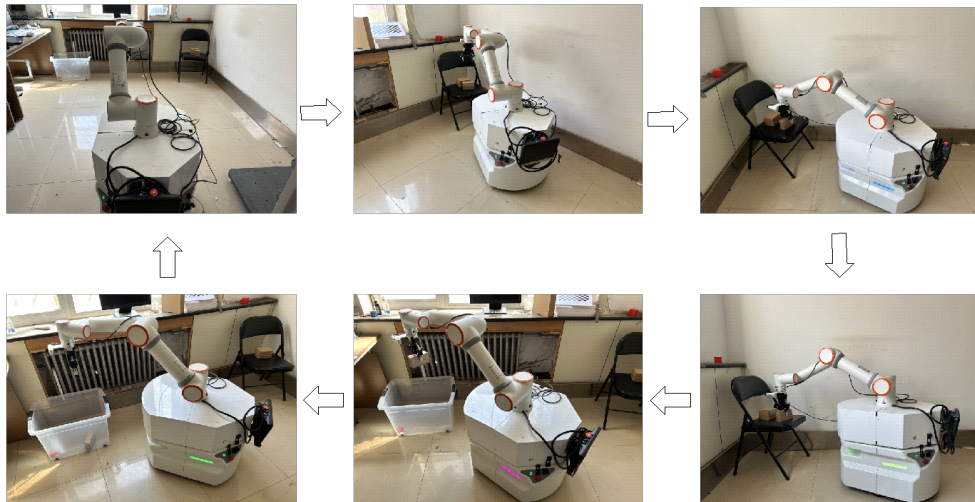
Fig. 15. Vision-based mobile manipulation for parcel grasping
